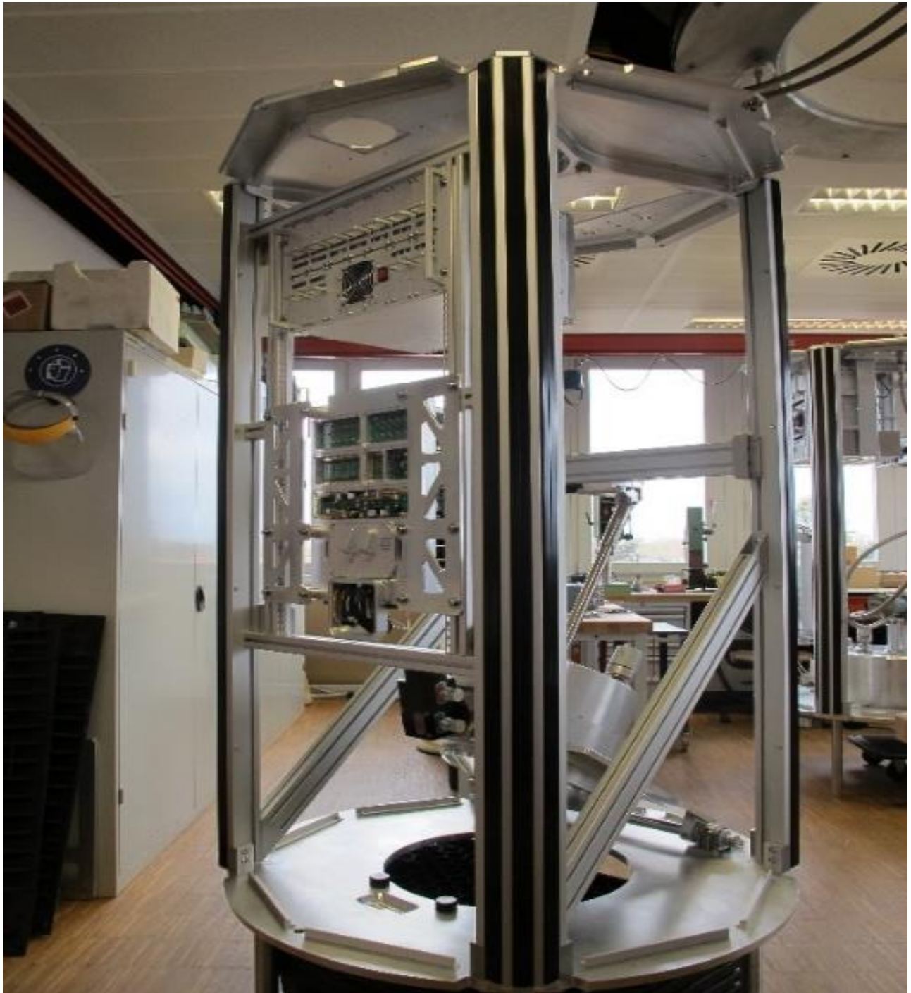
Figure 1: Picture of the UBB Rx in the laboratory. The feed points downwards and is automatically pulled up into the Rx box for storage. In the centre left is the highly integrated EDD front-end unit, which provides control, monitoring, RF conditioning and digitization.
